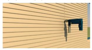
Commence installing cladding in accordance with manufacturer's installation instructions.
