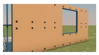
4. Provide for outer air space by adhering the Kingspan AIR-CELL Spacer Biscuits™ to the outer face of the Kingspan AIR-CELL® (approximately 3 Spacer Biscuits™ per square metre required).
