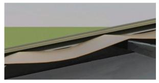
2. Allow a nominal 40 mm sag between purlins. If mesh is used, ensure that the mesh is installed loosely to allow for this sag.
