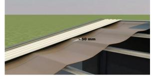
Overlap by 50 mm at joins and apply 72 mm reinforced foil tape to top of join. Alternatively allow 150 mm overlap when joins are not to be taped.
