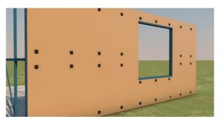
4. Provide for outer air space by adhering the Kingspan AIR-CELL Spacer Biscuits<sup>™</sup> to the outer face of the Kingspan AIR-CELL Insulshed<sup>®</sup> 50 (approximately 3 Spacer Biscuits<sup>™</sup> per square metre required, Kingspan AIR-CELL Spacer Biscuits<sup>™</sup> comes with a peel off self-adhesive backing).
