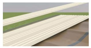
5. Fix roof sheeting by screwing through *Kingspan* **AIR-CELL** Insulshed<sup>®</sup> 50 to the purlins.
