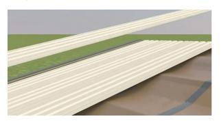
5. Fix roof sheeting by screwing through *Kingspan* **AIR-CELL®** to the purlin.
