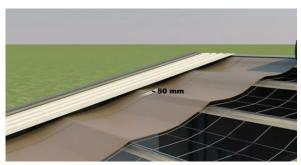
3. Overlap by 50 mm at joins and apply 72 to 100 mm reinforced foil tape to top of join. Alternatively allow 150mm overlap when joins are not to be taped.
