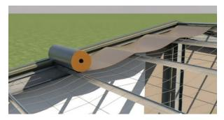
Lay Kingspan AIR-CELL® perpendicular to purlins ensuring a 25 mm overlap into the gutter.
