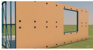
Provide for outer air space by adhering the Kingspan AIR-CELL Spacer Biscuits™ to the outer face of the Kingspan AIR-CELL (approximately 3 Spacer Biscuits per square metre required).
