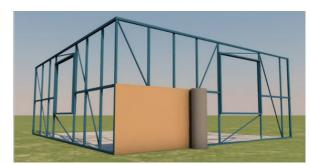
Fix Kingspan AIR-CELL loosely to the outside of frame leaving flexibility for Kingspan AIR-CELL to be dished onto the wall cavity.
